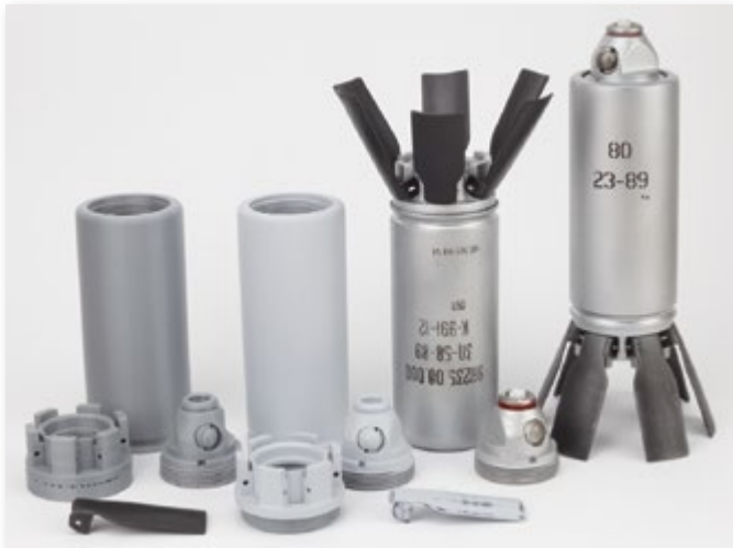
Figure 7. 3D printing multi-part 9N235 submunition replica for use in simulated benchmark photos and videos.
