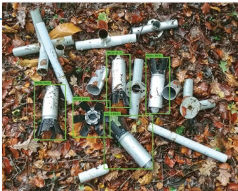
Figure 14. Test on low quality camera with motion blur using real FFE and 9N235/9N210 surrogate (replica) fabricated by Fenix Insight. Figure courtesy of Adam Harvey.
